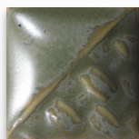
SW108 Green Tea under SW127 Olivine on EG006 Sparkle Black Engobe
