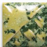
SW146 Aurora Green under SW127 Olivine on EG003 Brick Red Engobe
